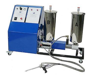
The LiquidShot 5 metering and mixing machine offers a reliable and economic solution for a wide range of resin dispensing applications, especially electronic potting. This machine exhibits a high degree of efficiency, accompanied by a portable floor mounted design. Proven piston pump technology allows for large shot applications typically dispensing between 100 to 250 ml per shot. High mixing ratios or large
